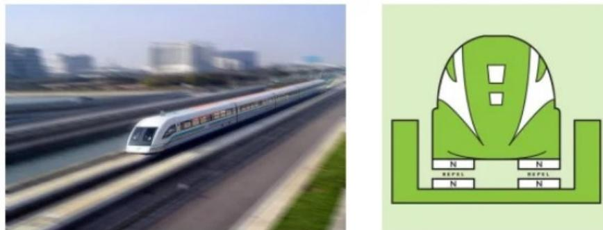
Let us study how the train levitates. There are permanent magnets on the bottom of the train, and electromagnets on the tracks. By providing power to the electromagnets, they generate a magnetic field, thus repelling the permanent magnets and applying an upwards force on the train. Because the magnetic field is stronger at shorter distances, for the same amount of power, the repulsion is stronger when the train is lower, and weaker when the train is higher.
